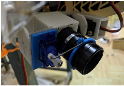
Figure 28: Automated Aperture Adjustment System
