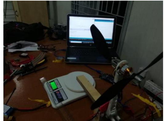
Figure 10: Coaxial Thrust measurement setup (1)
