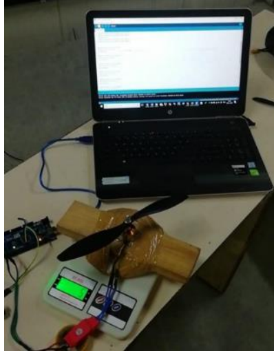
Figure 9: Single motor thrust measurement
